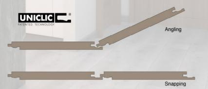
Unilin Uniclic is a patented glueless locking system used for our 91.5x15.2 SPC Vinyl planks. It works for both the long and short sides of the panel. It can be installed by angling or snapping the panels into each other, without the need for glue or nails. Uniclic guarantees a strong and seamless joint between the panels, thanks to its flexible lower lip and the contacts and spaces in the joint. Uniclic also ensures long-lasting stability and reduces unwanted creaking sounds.
